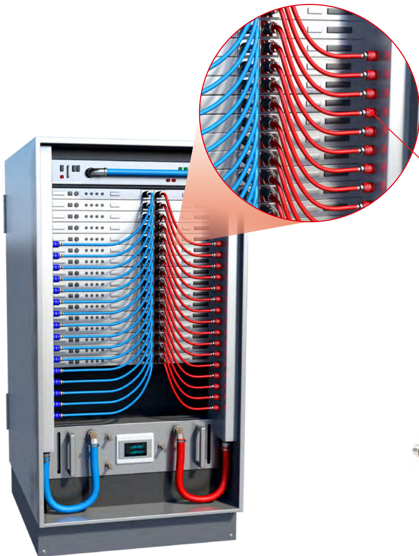
UQD Universal quick disconnect coupling
